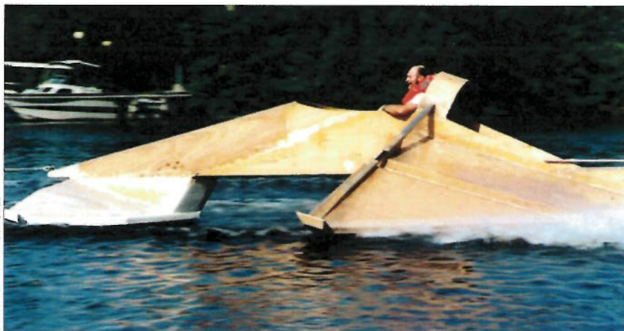
Left —Among the many unusual boats Schoell experimented with was this ground-effect machine prototype, where, as forward speed increases, aerodynamic lift is developed, separating the hull from the surface, which in this case is water. Right —Schoell's current fascination is with compact Rankine-cycle steam engines that are essentially silent and run on numerous types of fuel.
