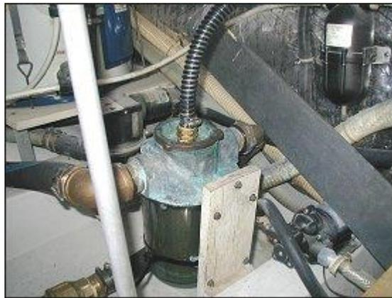
Fresh water flush plumbing - New fittings and hoses were attached to the raw water strainers and connected to a cockpit-mounted manifold to allow fresh water flushing of both mains and the genset.
