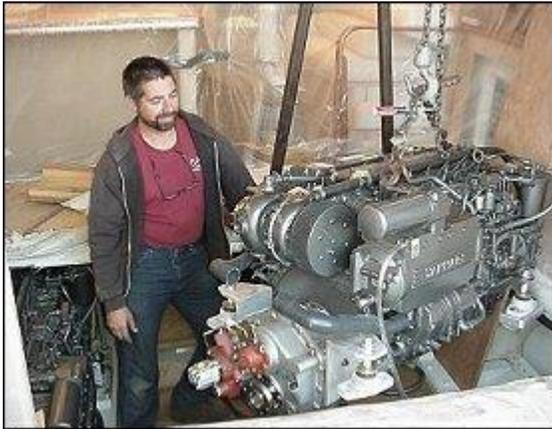
Here's Bill getting ready to position the new starboard engine. (Notice the bagging and other protection that protects the rest of the boat while the "dirty" work is being done).
