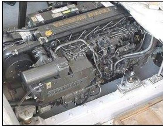
The port engine is roughed into place. Note the custom-made rear and forward mounting brackets. Both were fabricated at Seaboard. The existing stringer cap bracket (painted white and bolted to stringer) was reused to avoid major rework to the stringers.
