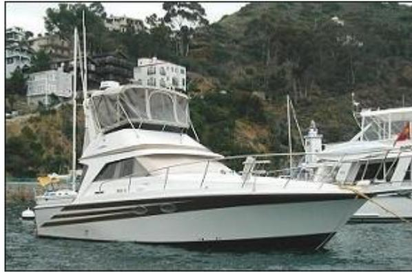
With a full load, BOSSEA displaced an estimated 19000 to 20000 pounds, and was capable of 22-23 knots at the top end in calm conditions. Top RPM achieved was approximately 2900 RPM, suggesting a modest
