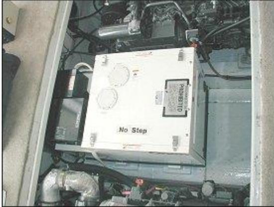
Generator is in - One of the last steps was the genset installation. Here it is with sound shield in place.
