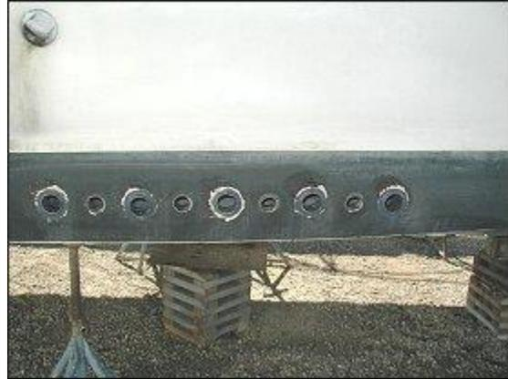
Enlarged exhaust - The external underwater exhaust ports had to be enlarged to take the greater capacity of the 6LYAs.
