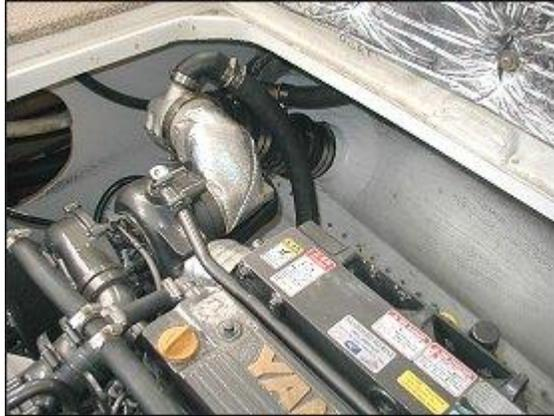
Enlarged exhaust - The neck into the built in muffler had to be enlarged also.
